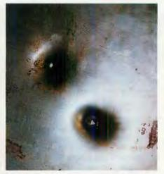
Fired at a 0.06-inch steel plate at 40 yards with Buck Shot, the Saiga-12K gave 50% penetration.
